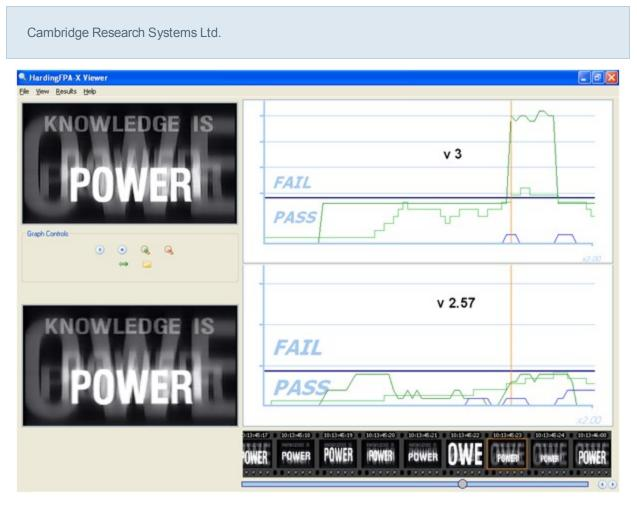
Most importantly of all, the Version 3 algorithms have been designed to be as format-agnostic as possible. Changes in file formats or codecs will alter the underlying video data even if these changes are not visually apparent. Here, the same video has been encoded at the same resolution using two different codecs. The absolute differences between the two images are shown in the third image as deviations from mid grey.
