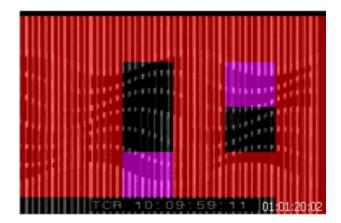
The mask data appears as a set of uniformly coloured tiles in the image which represent how long they have persisted in the image sequence. Spatial mask data only appears for stationary, regular patterns which lead to failure. Any spatial patterns which drift, or are not regular, or do not persist in the video long enough to trigger a failure are excluded.
