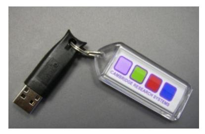
The HardingFPA HD must be licensed with a USB hardware protection key in order to run (see below).
