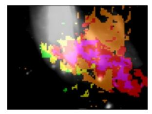
The colours represent the number of transitions which each pixel has experienced in the most recent second after allowing for motion. The analyser will issue a failure when more than one quarter of the image contains red or purple pixels. The same colour coding (shown below) is used for both luminance and red flash analysis.
