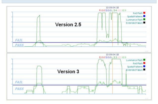
However, the results between the two versions will not be identical. The Version 3 algorithms will, in general, be more slightly more lenient to complex, rapid motion:
